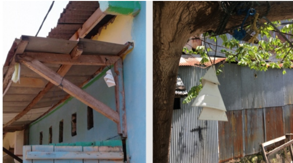
Image 4.1. Low-cost iButton temperature sensors housed in solar radiation shields in informal settlement communities in Makassar, Indonesia (Source: RISE Consortium).
